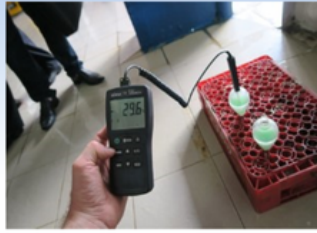
Evaporating temperature indicates approx. 15% H 2 O
