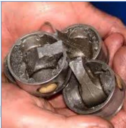
*The compressor fail as it is not designed to compress liquid refrigerant but refrigerant gas. The weak part in the compressor depends on the compressor design but is traditionally connecting rod, piston and valves.*
