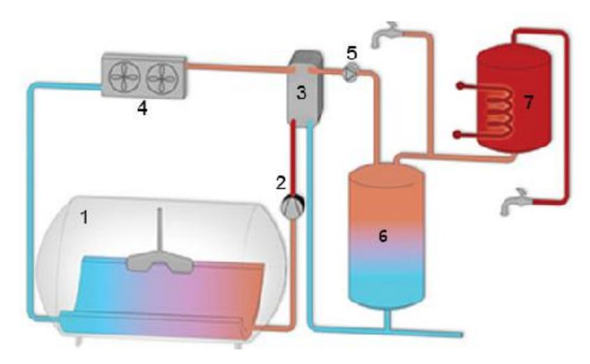
• Evaporator integrated in the milk tank
