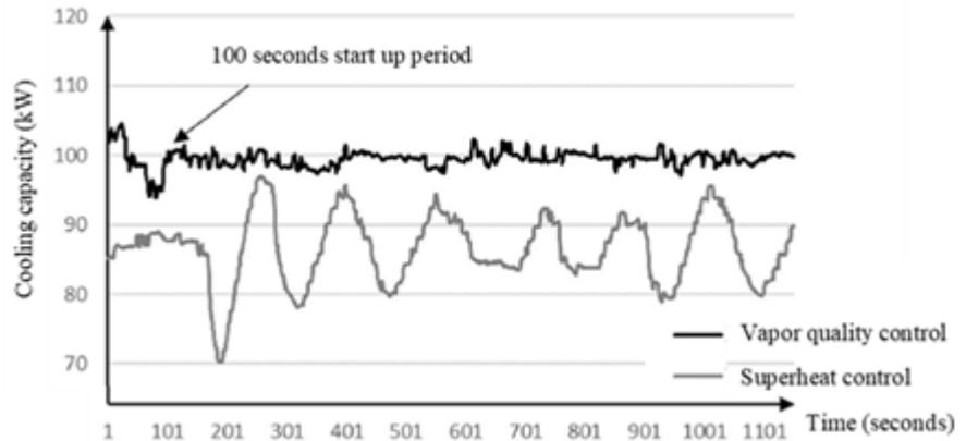
The graph shows that the variations in capacity are larger for the superheat control due to the relatively slow feedback from a temperature sensor used in superheat control. The Vapor Quality Sensor provides instant feedback and allows for frequent small actions.
