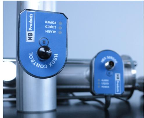
The working principle is capacitive which means, that in reality the sensor is a capacitor, and the fluid is the dielectric media. The total capacitance is measured, and the volume percentage is calculated based on the assumption that gas has a dielectric constant of 1 and the liquid has a higher value. The calibration covers the geometry and the dielectric constant of the liquid – this is found experimentally at operating temperature.
