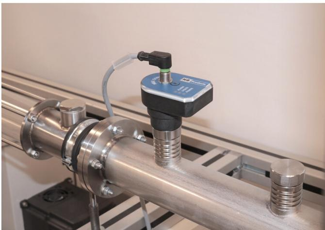
The Vapor Quality sensor can measure very small amounts of liquid in a gas flow. The sensor is designed and used for controlling evaporators which means there is little focus on accuracy. Normally the sensor is calibrated for dry gas only because this is what matters for the control system.
